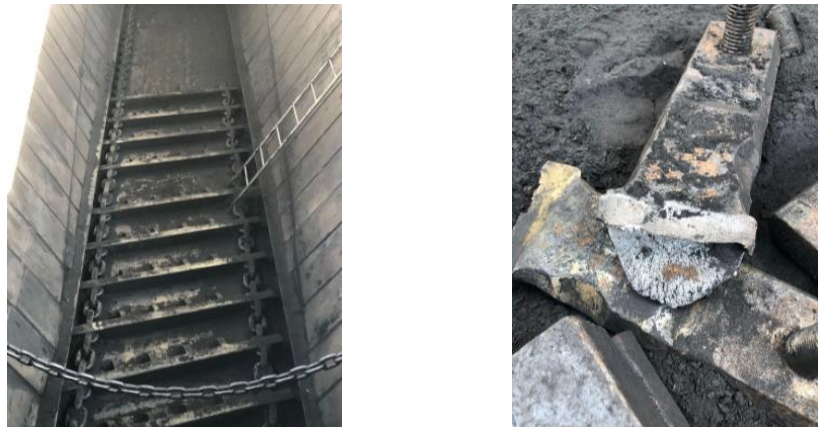
(a) Scraper conveyor's broken chain scene (b) Scraper fracture caused by broken chain
