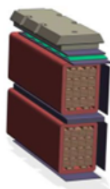
Figure 2. Overall structure of stator slot wedges
