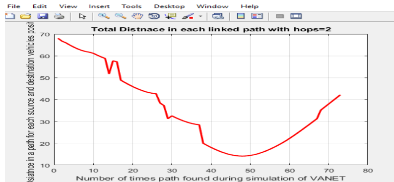
Fig.2. Simulated results of distance measurement between source and destination and their linked path for hops=2
