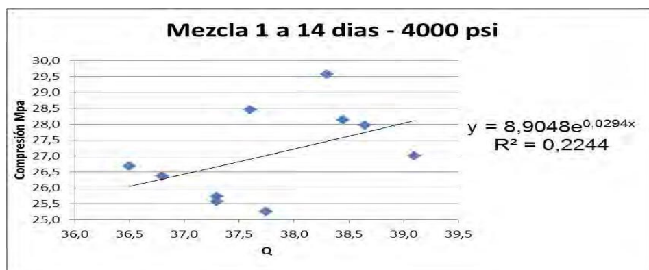
Figure 36. Trend Curve for Mixing 1 to 14 Days - 4000 psi
