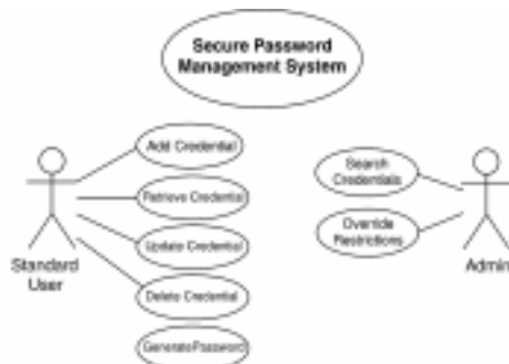
Fig. 1 Use case diagram of the password management system illustrating the interactions between the standard user and administrator roles with core system functionalities such as credential management, encryption, password generation, and role-based access control.
