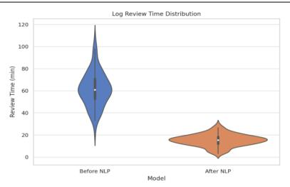
The log to root cause inference pipeline was hooked into Datadog anomaly alerts and Datadog could add anomaly context of the anomaly to triage tickets automatically. This made it possible to estimate the root cause, almost in real time, which was confirmed manually by SREs. This has reduced the average time of completion of RCA, from 66 minutes to 14 minutes.
